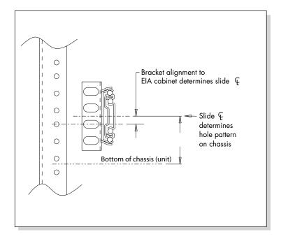
In some cases, one element of the slide installation is known, and this determines slide positioning.
