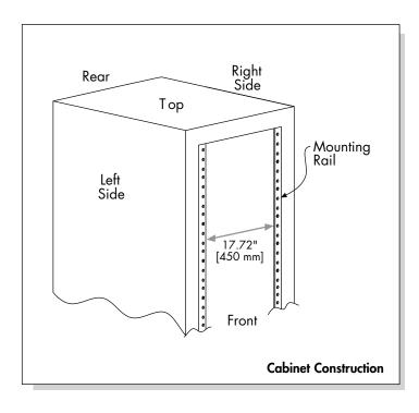
Most electronic cabinets/enclosures are based on dimensional guidelines as illustrated in the ANSI/EIA 310 Specifications.
