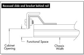
The drawings at left show several mounting configurations from an overhead perspective. This viewpoint demonstrates how to calculate chassis widths, evaluate slide thicknesses, and verify bracket installation.
