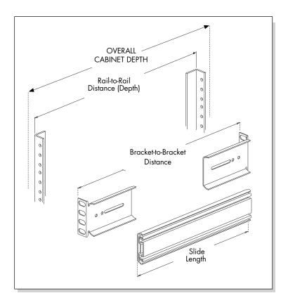
O Enclosure depth is measured from the front of the cabinet to the rear. It is greater than the mounting rail distance, which is measured from the front rail to the rear rail.
