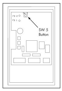
Figure 4.2 - Control Box Interior
