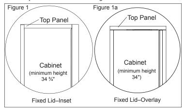
Build top panel according to desired inset or overlay layout and cabinet dimensions shown in figure 2.
