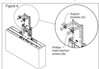
Verify support brackets are symmetrical in relation to the center line and 8-13/16" apart as shown in figure 5.
