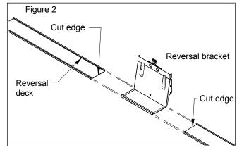
4. Loosen the Phillips screw on the reversal bracket and insert decks, cut edge in (fig. 2).
