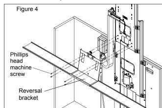
6. Insert (4) Phillips head machine screws through the slots of the reversal bracket and into the four threaded holes located near the bottom of the CB Lift-050 and securely fasten (fig. 4).
